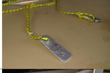
Attach this link to the aft-most hole in the stem fitting and retain it with the spring pin. The mast is now secure.
