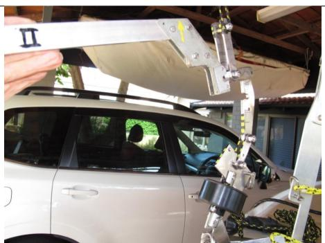
Take the strain, and remove the split pin.
