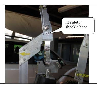
When the linkage has gone over centre the linkage will be secure for the moment.
