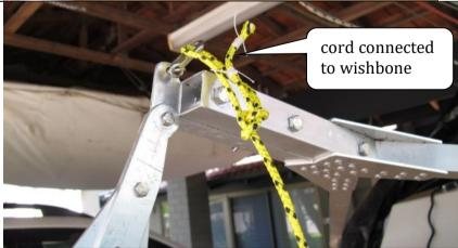
The mast will be supported at the bow by an aluminium link. Disconnect this link from the bow fitting (store the spring pin in the other hole in the bow fitting). Swing the frame up and over the cabin, paying out the yellow cord that connects the link to the pulley, then pay out the red/white line from the pulley, until it comes up against the stop knot. Shackle the other yellow cord to the (lower) saddle on the
